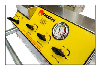
A simple lever controls the movement of the lifter from 0° though to 90°
